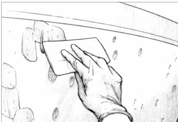
Figure 4-7 Trowel thickened fairing compound into the blister cavities with a plastic squeegee.
