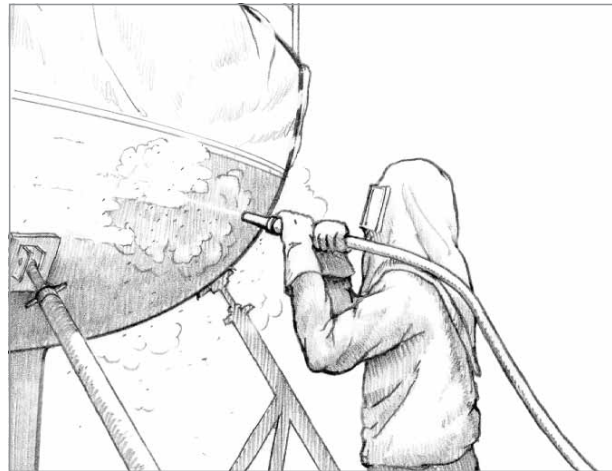
Figure 2-3 Sandblasting is a common method of opening blisters and abrading the hull.
