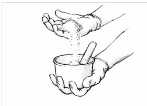
Figure 6-7 Blend in small handfuls or scoops of the appropriate filler until the desired consistency is reached.
