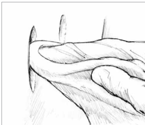
Figure 4-1 Wipe the cavity clean with alcohol and repeat until the laminate is dry to the touch.
