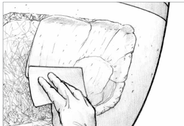
Figure 4-12 Apply a layer of epoxy/406 thickened to a mayonnaise consistency.
