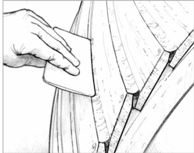
Figure 5-9 Fill the wet-out seam with thickened epoxy
