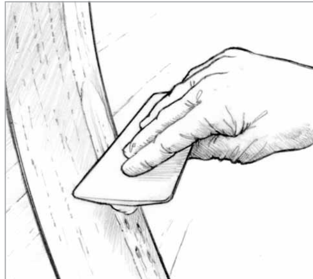
Figure 3-5 Fill the remaining voids with fairing compound.
