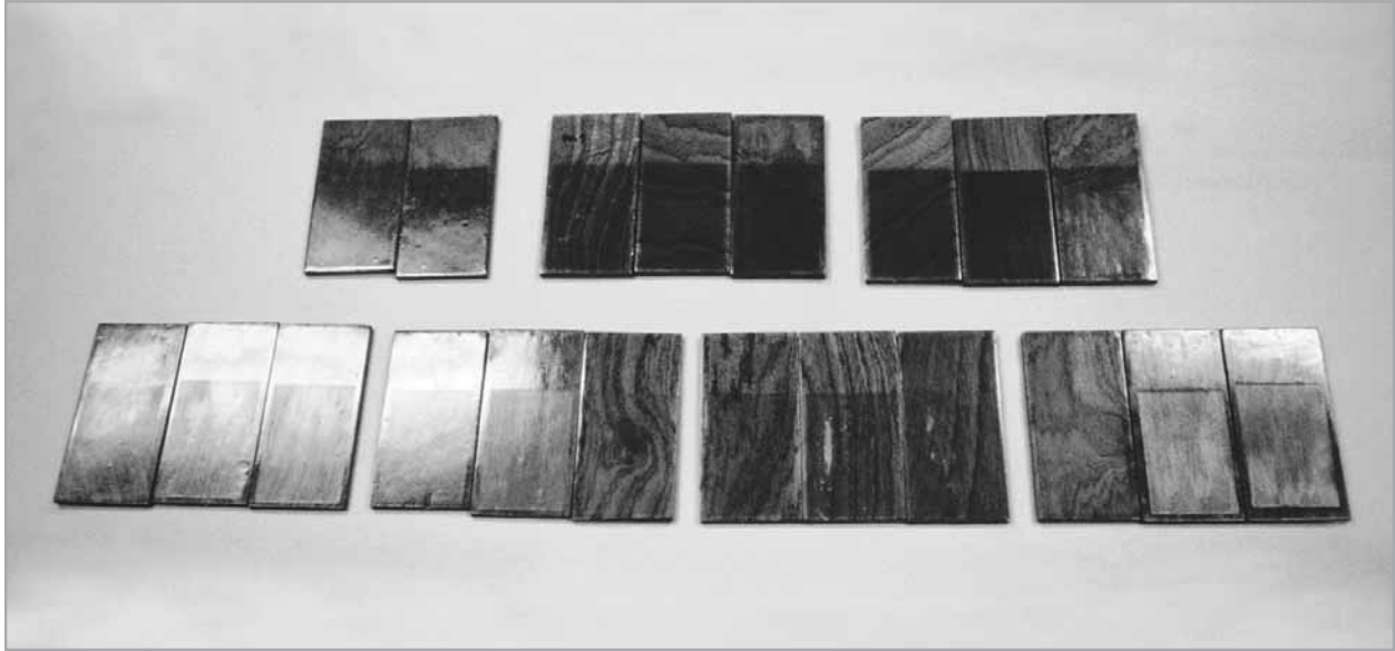
Figure 7-2 UV test samples after 3600 hours in weathering machine.
